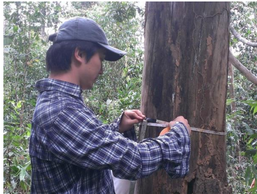
Figure 2: Measurement of diameter using a diameter tape and a pole
