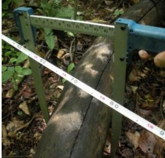
**Figure 7: Use of calipers to measure the diameter of lying deadwood along line transect**
