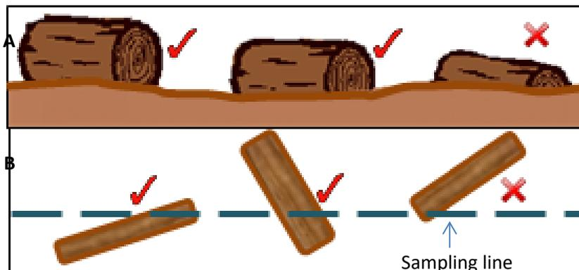
**Figure 8: (A) Schematic of which deadwood should be measured. The first two logs should be measured because they are more than 50% above ground, but the third log should not be measured. The horizontal line represents the soil surface. (B) Schematic of which deadwood should be**
